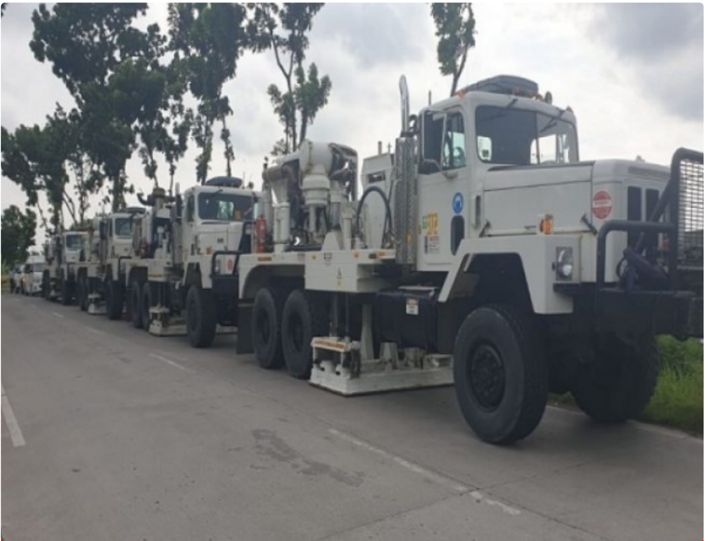
Survey Seismik 2D Vibroseis/foto: dok Pertamina
